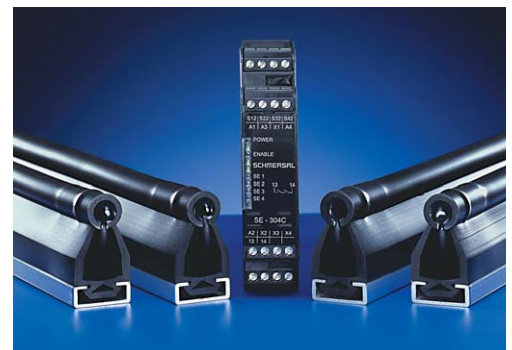
Image 4: Safety edges with optoelectronic operating principle: an infrared sensor detects the activation of the rubber profile.
