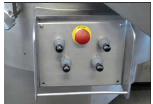
Image 4: The joystick switches installed on the control panel provide for an intuitive operation of the machine
